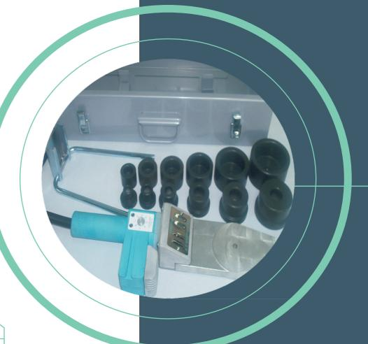
Special kind of additional tools are heating saddle welding sockets.
